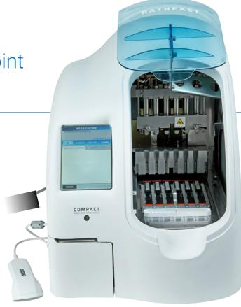
**Principle and Precision** PATHFAST TM is a fully automatic immunoassay analyzer, which combines the progressive chemiluminescence technology with the patented Magtration TM technology. Small sample volumes can be detected with high accuracy and precision. The device and the reagent strips provide optimum sensitivity. The results are perfectly reproducible and correlate outstandingly with lab analyses.
