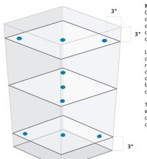
**Measuring Uniformity** Over two periods, uniformity data is collected from nine different points in the freezer door opening.
