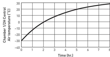
Conditions: AT 35°C, no load, measured at center of chamber
