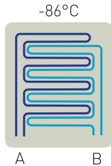
Dual Cooling System in Upright Freezers (MDF-U500VXC & MDF-U700VXC)
